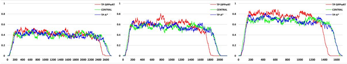
Figure 4: Number of tasks executed per second in a moving 100-second window ( $t - 100, t$ ] (that is, throughput at time  $t$ ) as a function of time  $t$  for different MAPD algorithms. Left:  $v_{task} = 0.50$  m/s. Middle:  $v_{task} = 0.75$  m/s. Right:  $v_{task} = 1.00$  m/s.
